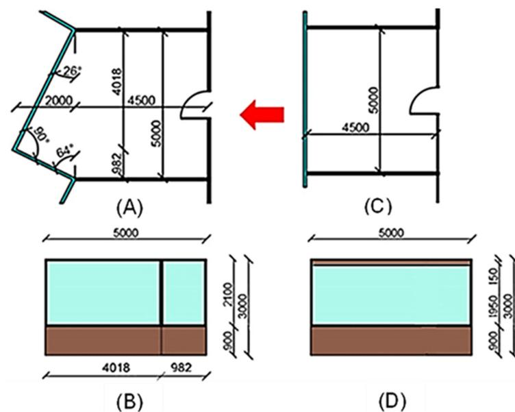
**Figure 1.** (A) A diagram illustrating an office room plan with multi-angled façade solutions. (B) A façade system designed with multi-angled façade. (C) An office room layout featuring a flat façade. (D) A design representation of a flat façade.
