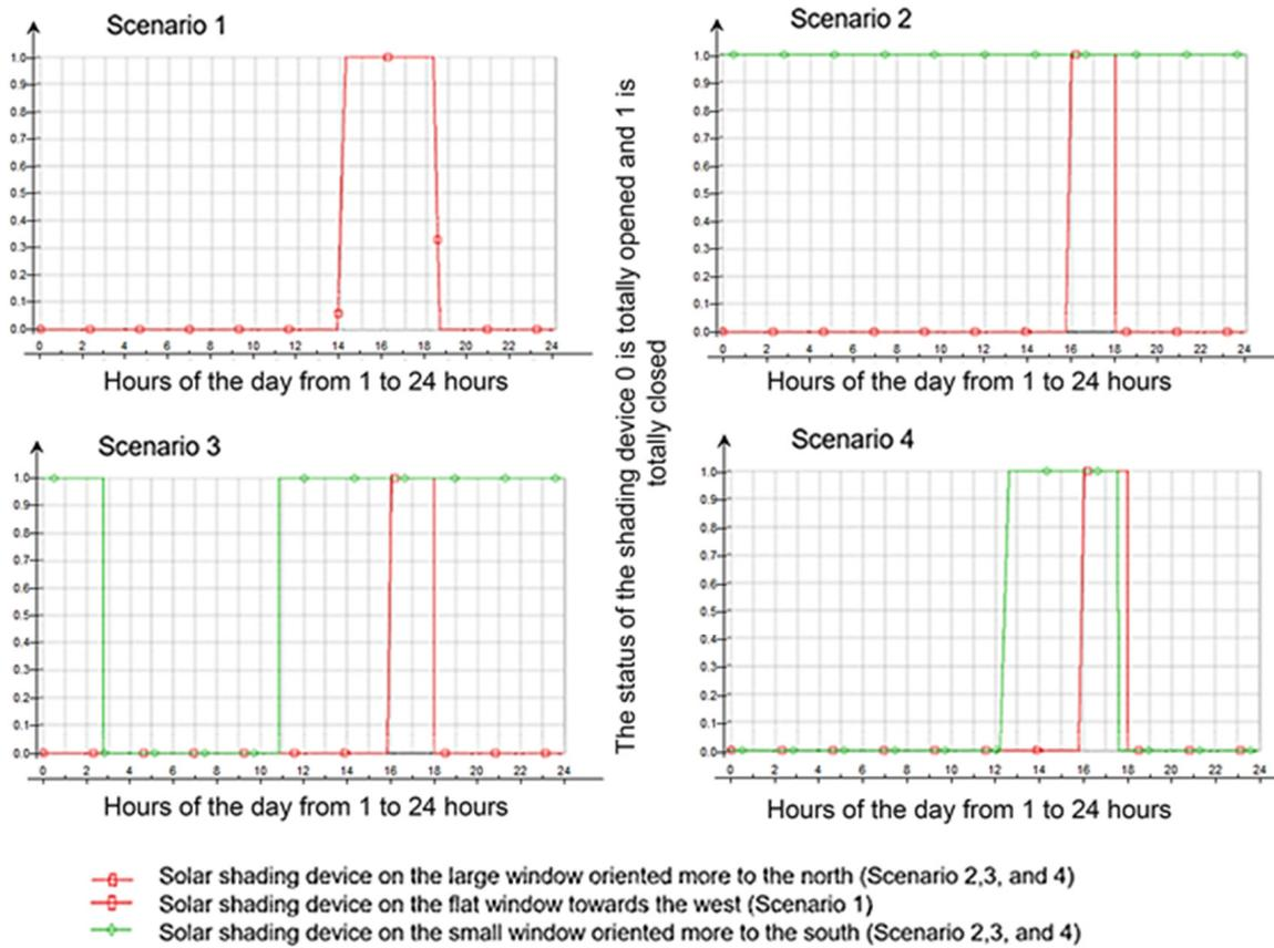
Figure 8. Scenarios in which the shading devices are closed on a day in the middle of July.
