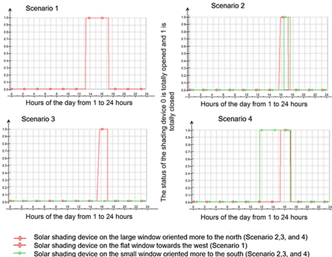
Figure 10. Scenarios in which the shading devices are closed on a day in the middle of March.
