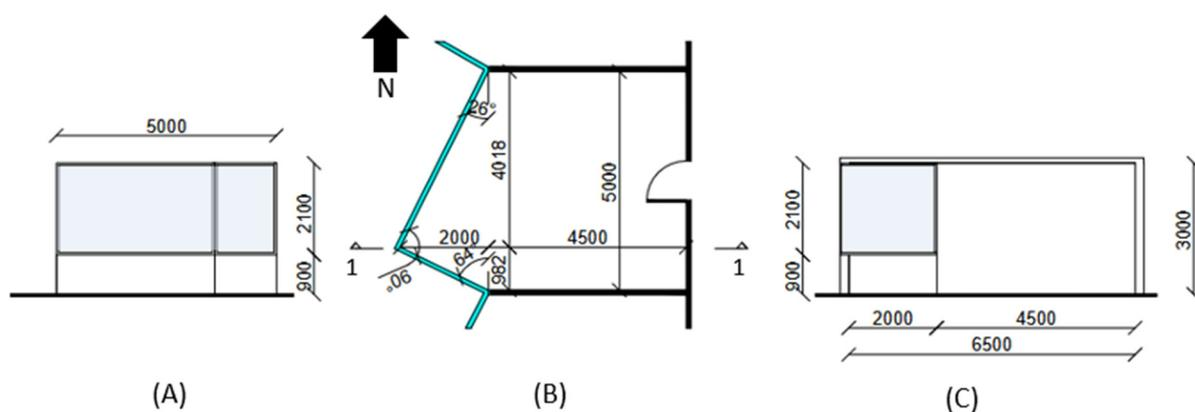
**Figure 7.** (A) The multi-angled façade system. (B) Floor plan of an office room featuring a multi-angled façade system, where the larger section faces north and the smaller section faces south. Dimensions are included to illustrate the relationship between the façade extension and the overall room layout. (C) Section view (sec 1-1) through the office room.
