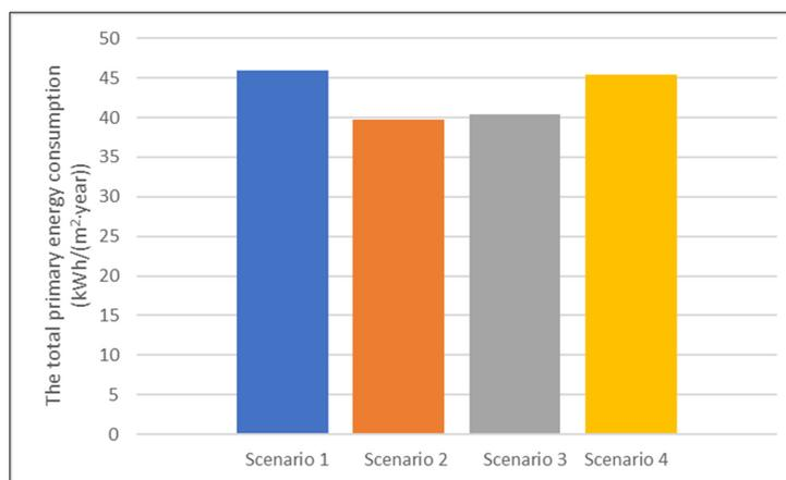
**Figure 11.** The simulation results present the total primary energy consumption for all four scenarios in compliance with BR15.
