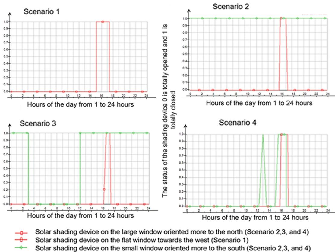
Figure 9. Scenarios in which the shading devices are closed on a day in the middle of May.
