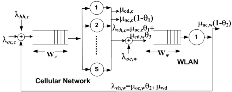
Figure 7.2: The two stage open queuing system considered
