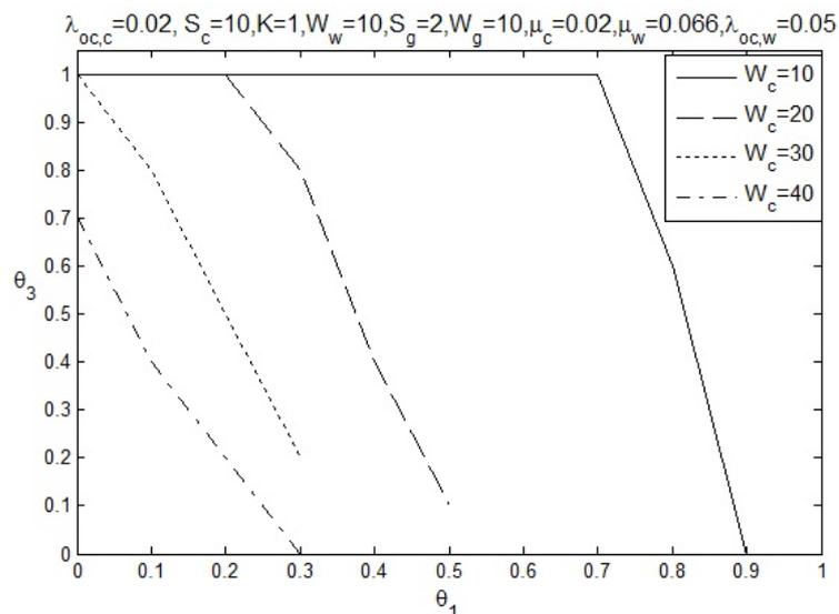
Figure 9.6: Downward vertical handover probabilities for different  $W_c$
