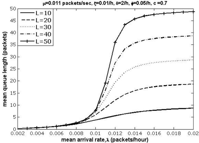
Figure 5.20: MQL results as a function of mean arrival rates for different queue capacities
