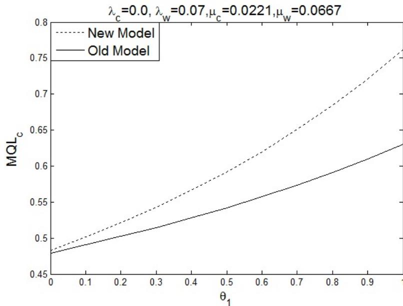
Figure 8.4: Effect of the feedback streams on  $MQL_c$  for scenario 1
