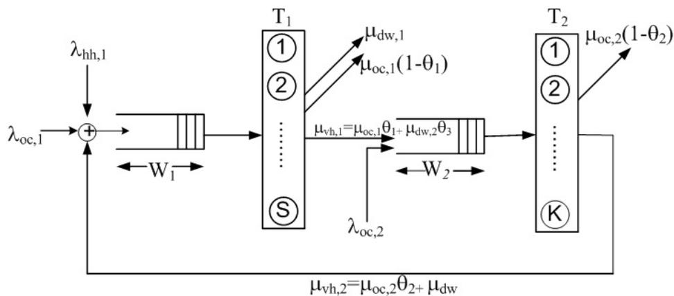
Figure 6.2: The two stage open queuing system considered
