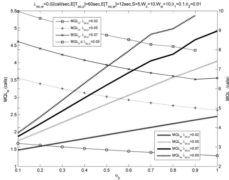
Figure 7.9: The MQL results for both Cellular ( $MQL_c$ ) and WLAN ( $MQL_w$ ) as a function of  $\theta_3$  with various  $\lambda_{oc,c}$  values.
