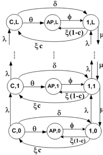
Figure 5.3: The state diagram of the proposed WLAN
