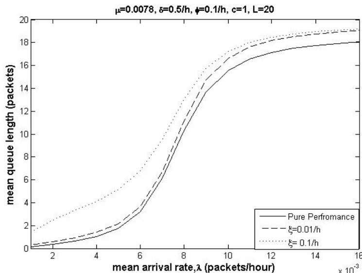
Figure 5.4: MQL results for systems with various channel failure rates
