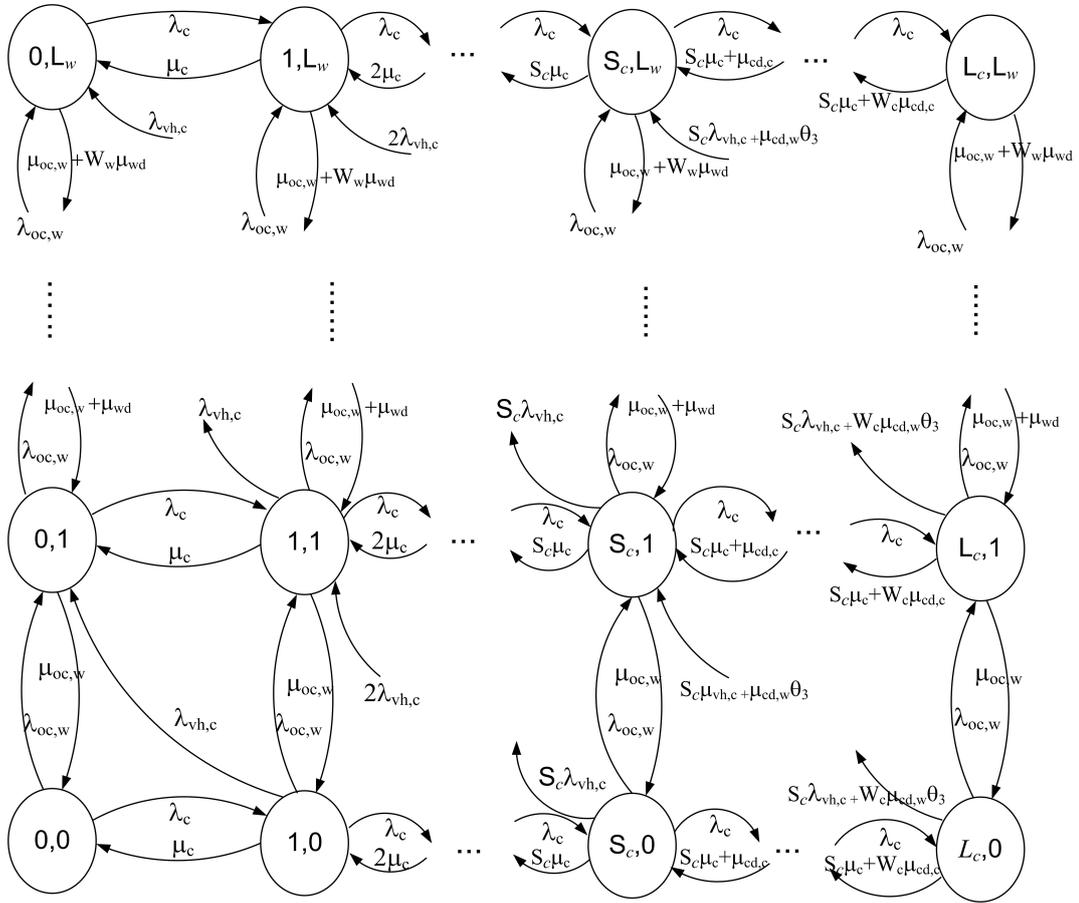
Figure 9.2: The stage diagram queuing system considered for downward vertical handover
