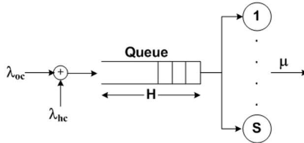
Figure 4.1: The model considered for a cellular network
