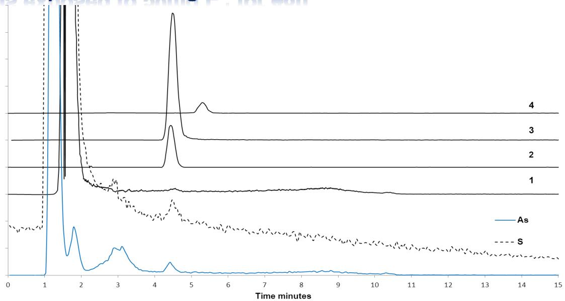
1 GSH (308), 2 DMAS<sup>V</sup>-GS (444), 3 Reduced PC<sub>2</sub> (540) and 4 Oxidised PC<sub>2</sub> (538), As and S signals from HR-ICP-MS
