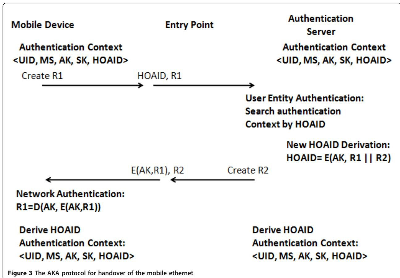
instead of sending the UID, the mobile device will initiate the authentication protocol by sending the HOAID and the R1 as the first message in Figure 3.
