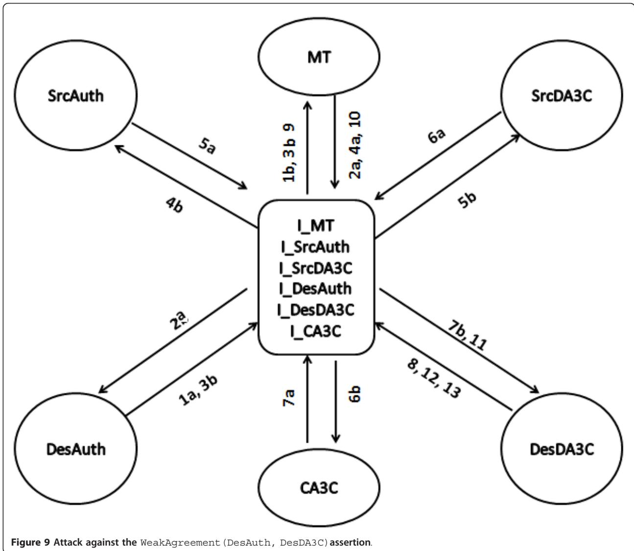
from message 8, the intruder impersonates the DesAuth and completes the protocol's run. Therefore, the discovered attack could be interpreted as follows: the DesDA3C believes that it has successfully completed the run with the DesAuth. However, in reality it was with the intruder acting as the DesAuth.
