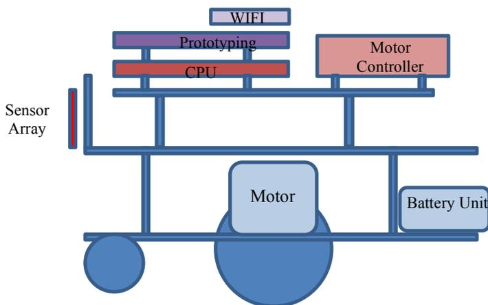
Fig. 2. Schematic diagram of the baseline robot
