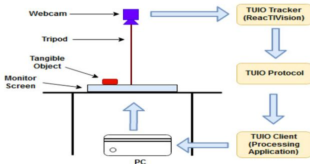
Fig. 4. Hardware setup and software architecture used for TangiNet
