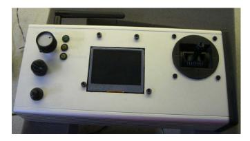
Fig. 6 Ground Control Unit with joystick for arm articulation and system locomotion.
