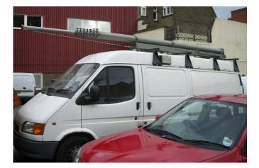
Fig. 3 Vehicle used by Metropolitan Police Force for capturing elevated images.
