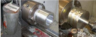
Fig. 7 Turning down process.
