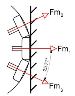
Fig. 14 Magnetic forces on flat vertical surface.
