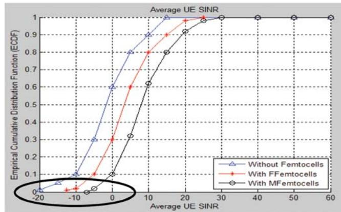
Figure 16. SINR of mobile UEs without & with FFemtocells/MFemtocell
