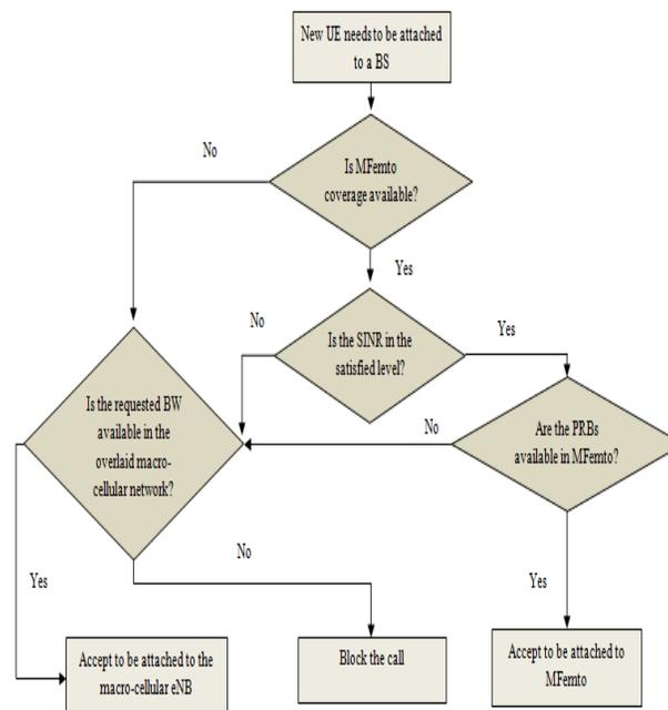
Figure 12. New connected UEs case 1
