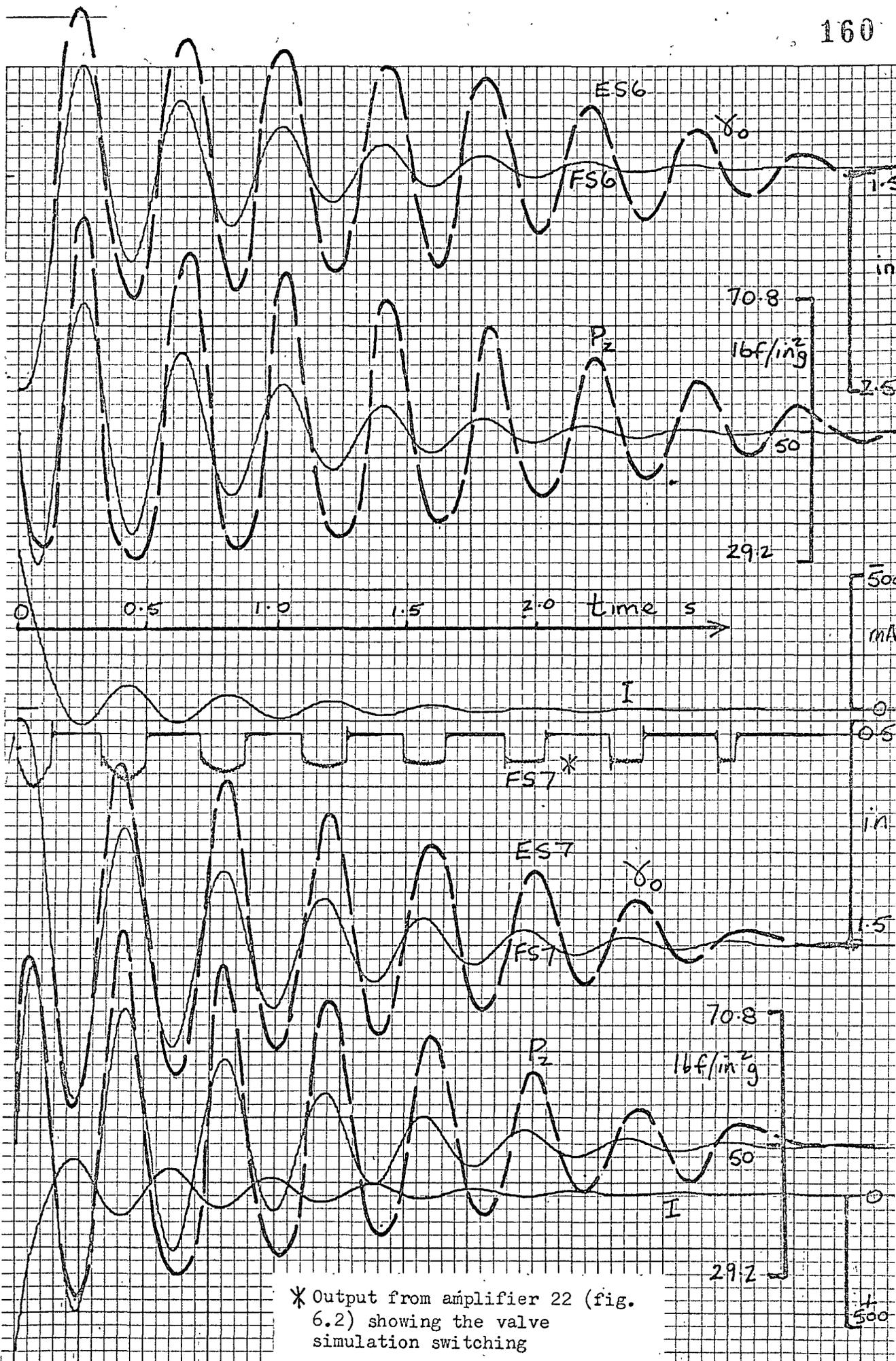
\* Output from amplifier 22 (fig. 6.2) showing the valve simulation switching
