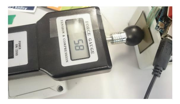
Figure 7.10: Using a calibrated force gauge to measure dynamic friction
