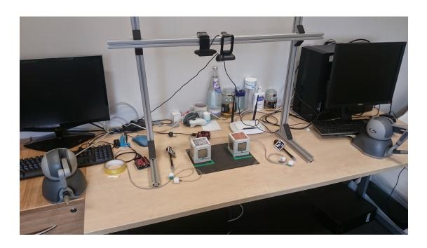
Figure 7.13: Setup of the study: two cubes, two webcams, two Phantom Omni, two PC with two screens, two pairs of GSR sensors and two styluses with AR markers.
