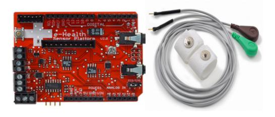
Figure 7.7: e-Health GSR sensors for Arduino
