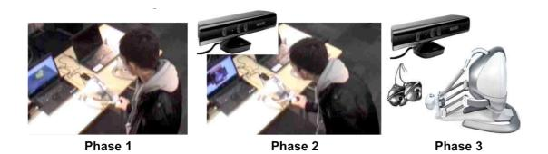
Figure 6.1: Experimental setup showing the three different phases. Phase 1 (left photo) participant interacting with the robot normally. Phase 2 (middle photo) participant trying the robot and a 3D camera (Kinect). Phase 3 (right photo) participant using 3D camera to control the robot to play a bell.
