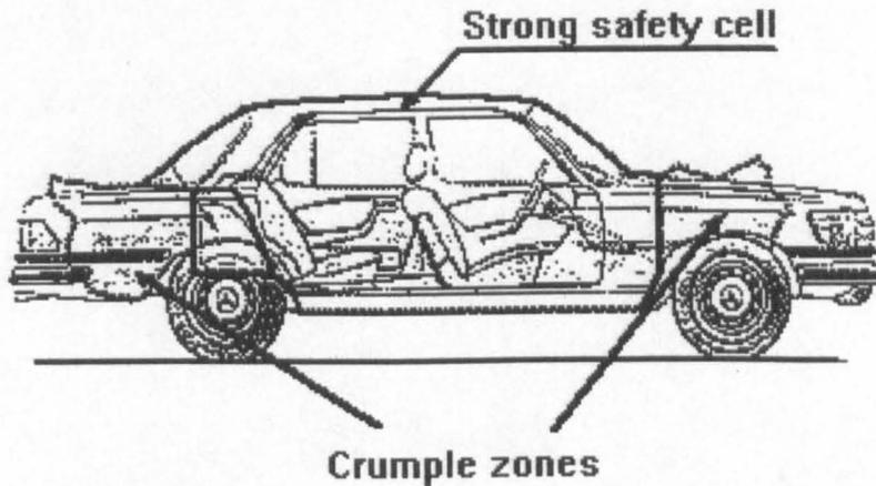
**Figure 4.3 Vehicle safety cell and energy absorbing structure [4.4]**
