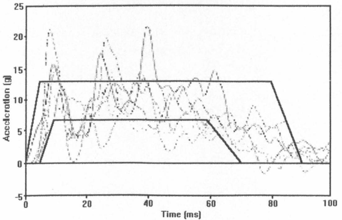
**Figure 13.16 Lateral acceleration of target vehicle [13.1]**
