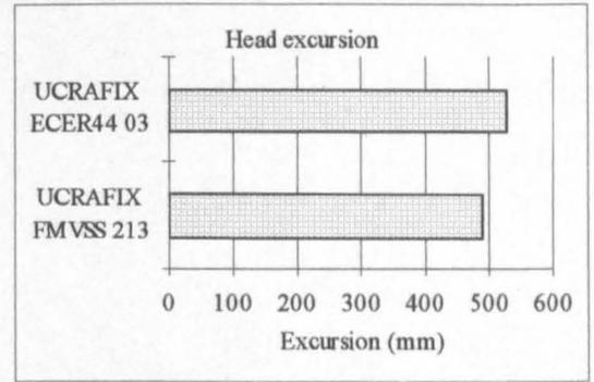
**Figure 11.37 P3 manikin excursion in New Zealand side impact test**
