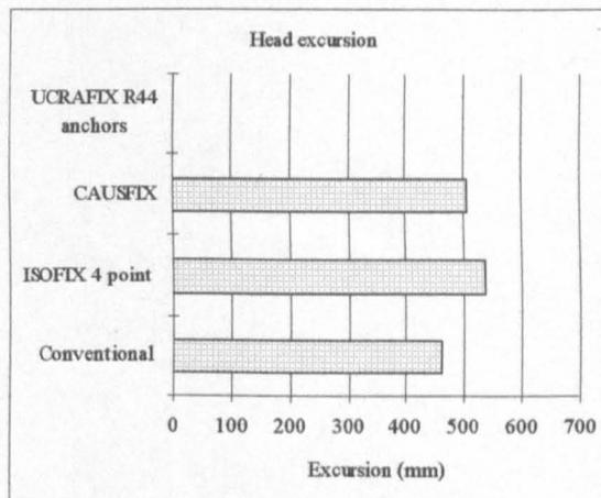
**Figure 11.52 Head excursion (std set up) P3/4 manikin**
