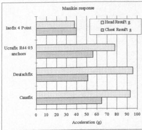
**Figure 11.54 Manikin accelerations rear facing Group 1 CRS**
