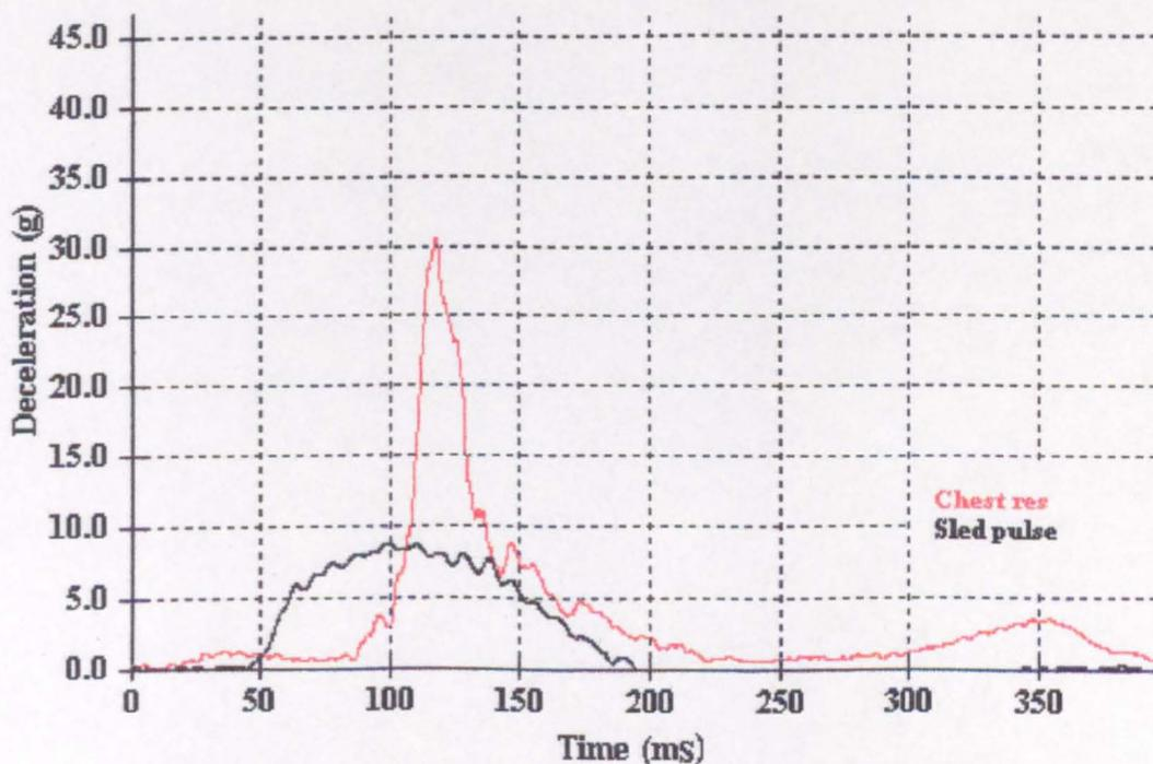
Figure 13.27 Occupant response in fixed panel test (T3337)
