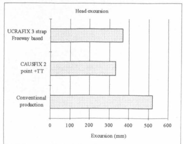
Figure 11.33 Head excursion (std set up) P3/4 manikin
