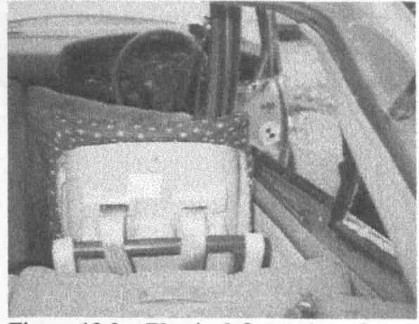
**Figure 13.9 Plastic deformation of vehicle side structure<sup>1</sup>**
