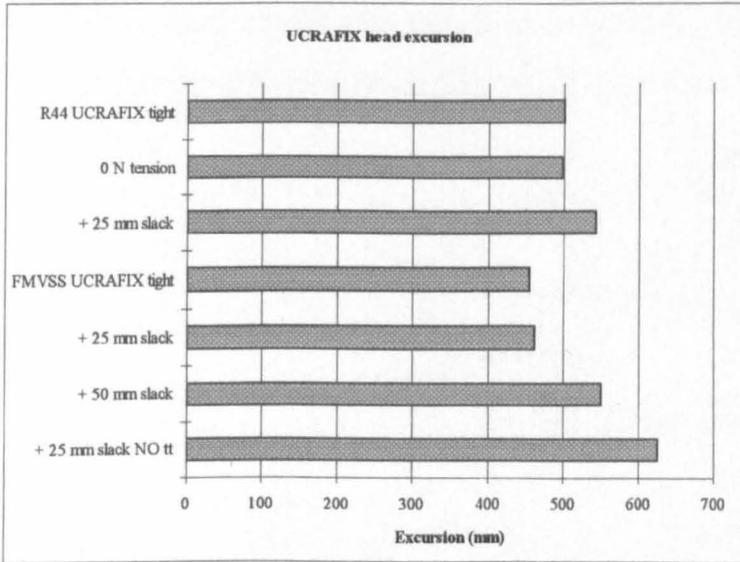
**Figure 11.26 The effect of slack on Ucrafix head excursion ECE R44 vs FMVSS 213 anchor positions**
