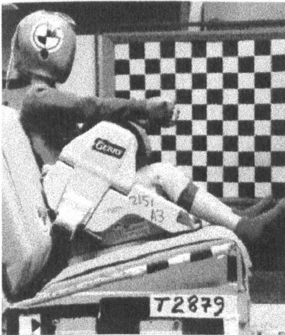
**Figure 6.8** Shield type restraint
