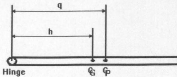
To minimise the load on the hinge, it is necessary to strike the 'intrusion panel' at the centre of percussion (C of P), at this point  $\sum$ moments about it = 0.
