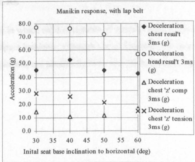
**Figure 12.65 Resultant deceleration levels, Lap belt retention**
