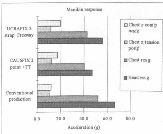
Figure 11.32 Manikin accelerations (std set up) P3/4 manikin
