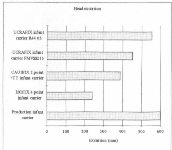
**Figure 11.60 Manikin excursions from centre line of test seat.**
