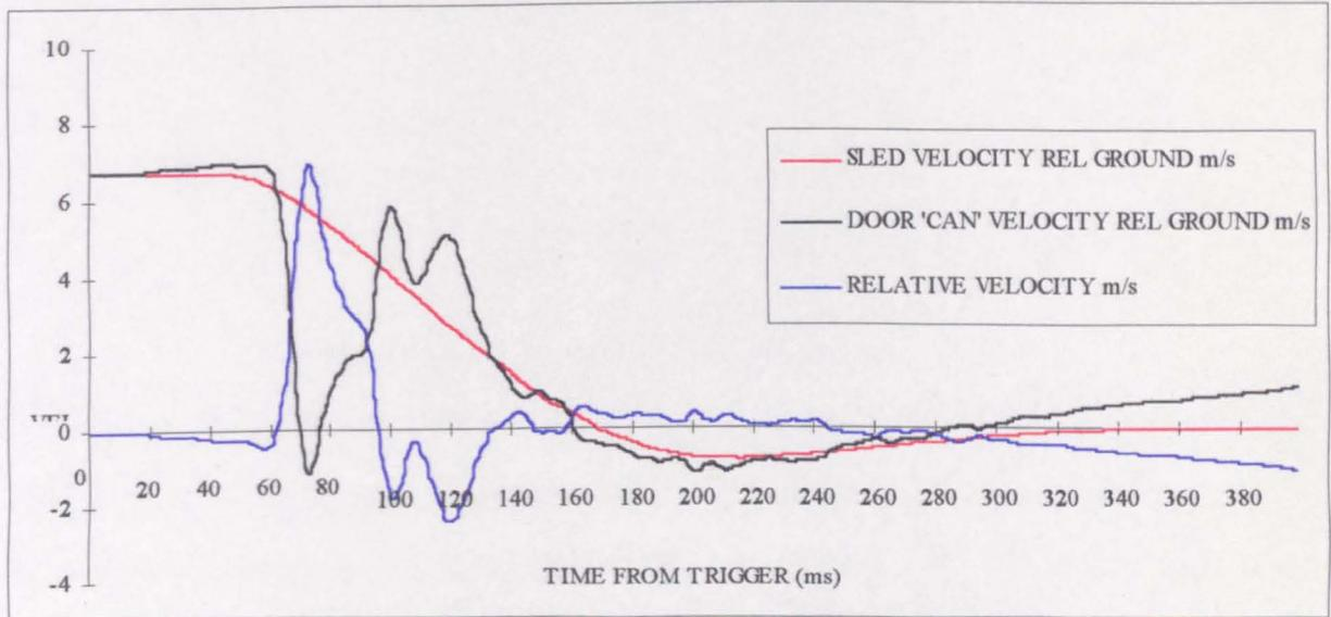
**Figure 13.24 Sled and 13 kg panel velocities (T3159)**
