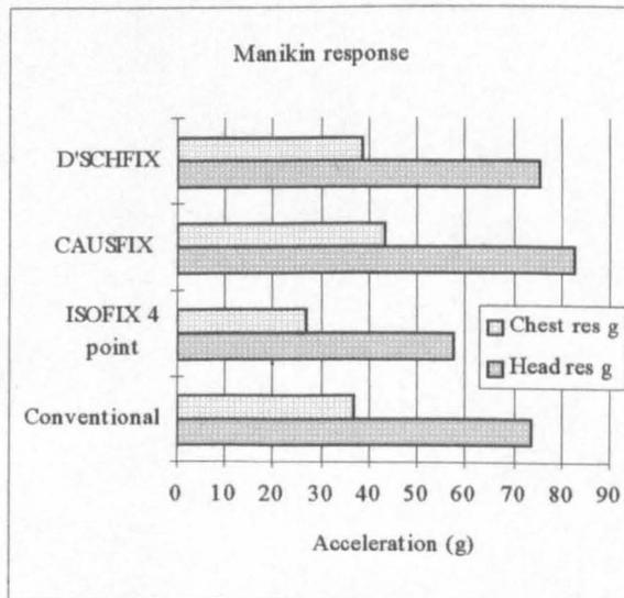
**Figure 11.42 P3 manikin response in rear impact**
