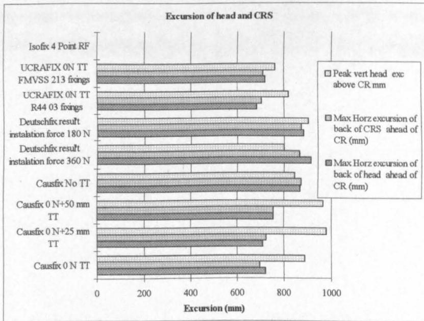
**Figure 11.58 Effect of slack on manikin and CRS excursion**
