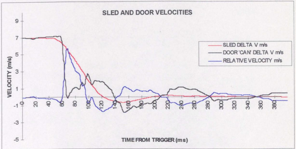
Figure 13.33 Sled and 30 kg panel linear velocities
