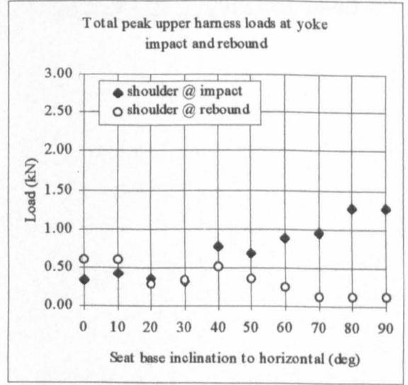
**Figure 12.56 Upper section loads at harness yoke behind shell**
