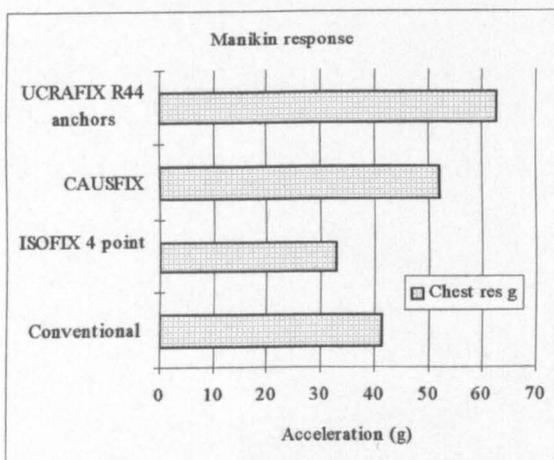
**Figure 11.51 Manikin acceleration (std set up) P3/4 manikin**
