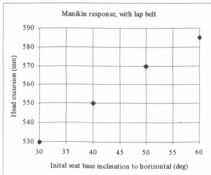
Figure 12.64 Head excursion, Lap belt retained CRS
