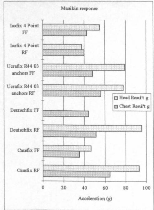
**Figure 11.55 Resultant accelerations Rear Vs forward facing**
