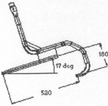
**Figure 11.3 Isofix (Unifix) 4 point CRS dimensions**
