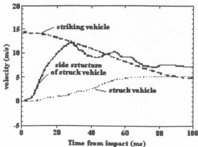
Figure 13.19 Typical velocities of struck and striking vehicles
