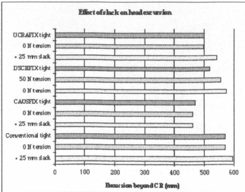
**Figure 11.23 Effect of slack on head excursion**
