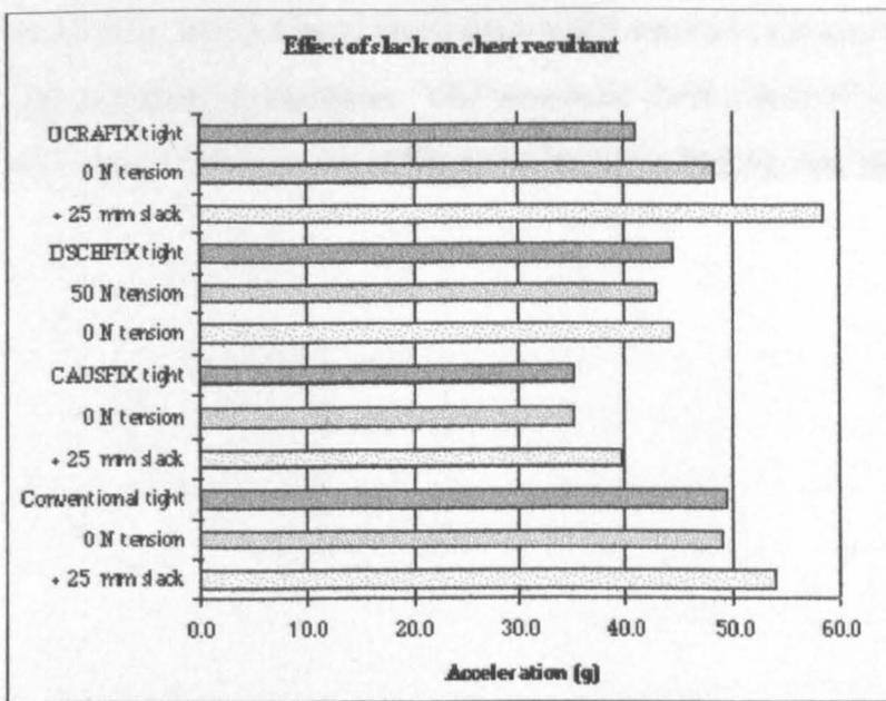
**Figure 11.24 Effect of slack on chest resultant acceleration**
