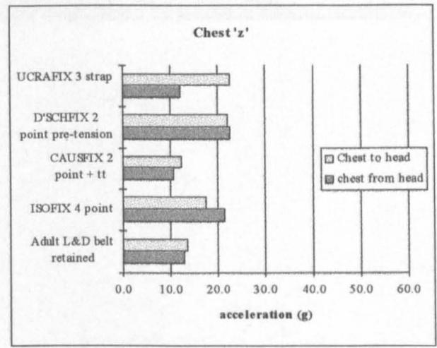
**Figure 11.22 Chest accelerations (ECE R44 limit 30 g chest to head) P3 manikin**
