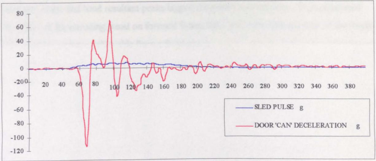
**Figure 13.23 Sled and 13 kg panel deceleration (T3159)**
