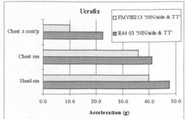
**Figure 11.20 Accelerations, ECE R44 vs. FMVSS 213 anchors**
