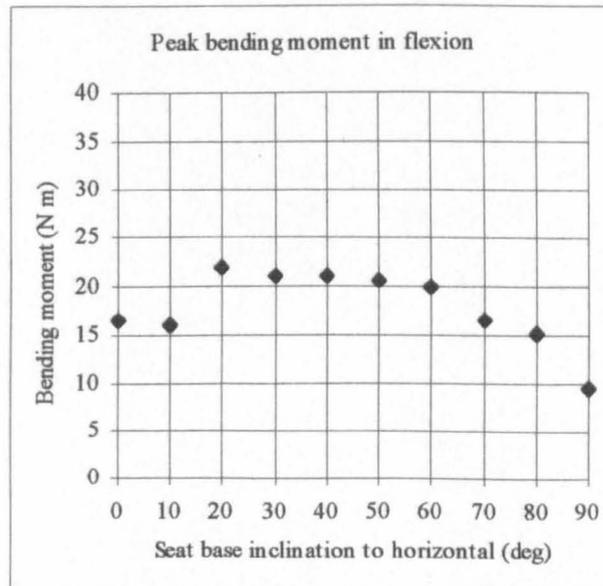
**Figure 12.54 Peak bending moment at atlas axis**
