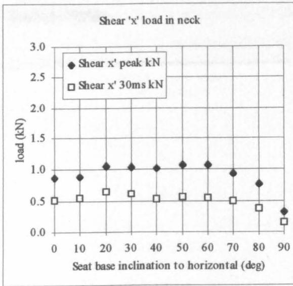
**Figure 12.52 Peak shear load at atlas axis**
