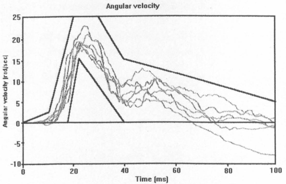
**Figure 13.15 Angular velocity of vehicle side structure with respect to vehicle frame of reference [13.1]**
