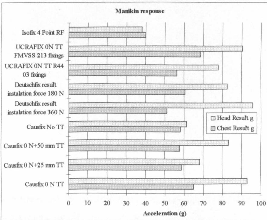
**Figure 11.57 Effect of slack on manikin acceleration response**
