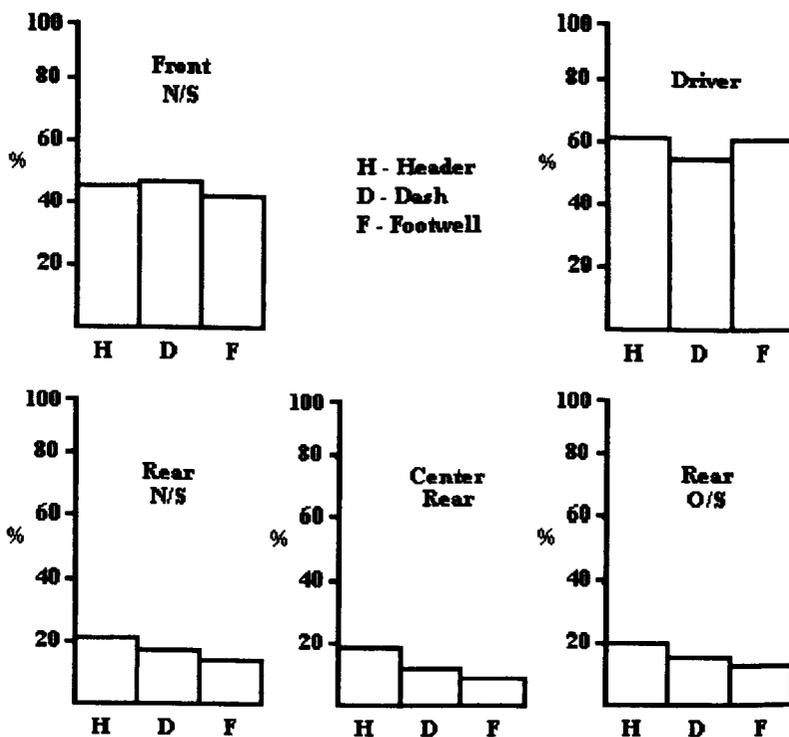
Figure 3.14 Seating position with respect to frequency of intrusion N=229 UK vehicles [3.7].
