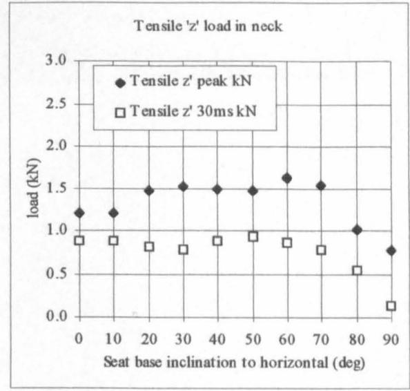
**Figure 12.53 Peak tensile load at atlas axis**
