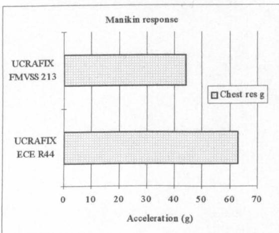
**Figure 11.53 Manikin acceleration ECE R44 03 Vs FMVSS 213**
