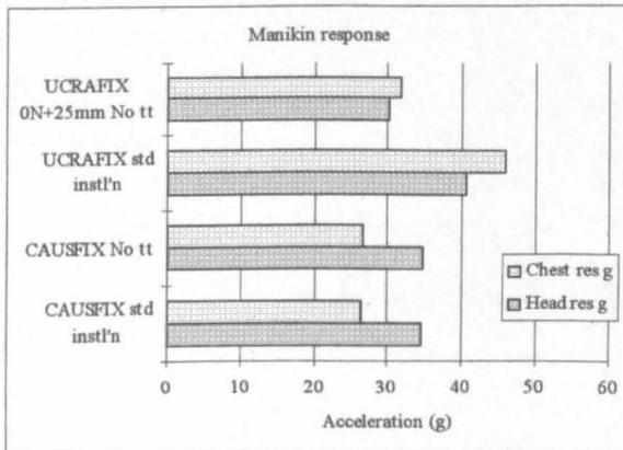
**Figure 11.40 Effect of tt deletion on acceleration levels P3 manikin in New Zealand side impact test**
