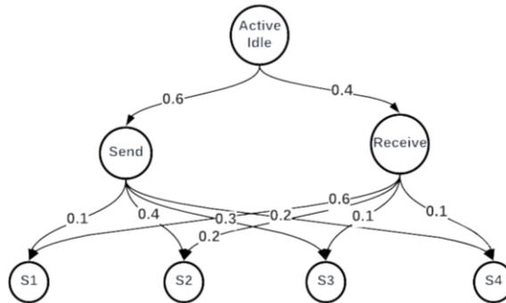
**Fig. 1.** Balancing Tx (Send) and Rx (Receive) states using HMM
