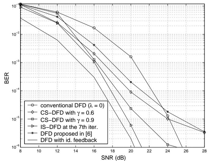
Fig. 4. BER performance comparison of the proposed decision feedback detectors (DFDs) with conventional DFD, DFD in [6] and ideal feedback DFD when channel length  $P = 12$ .
