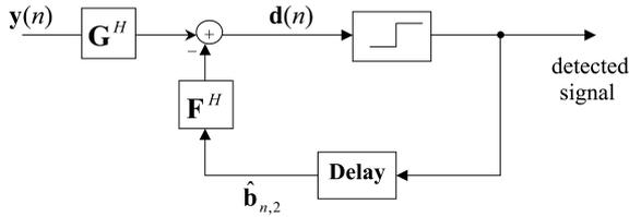
Fig. 1. Block diagram of decision feedback detector.
