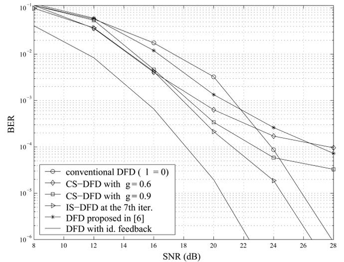
Fig. 3. BER performance comparison of the proposed decision feedback detectors (DFDs) with conventional DFD, DFD in [6] and ideal feedback DFD when channel length  $P = 6$ .
