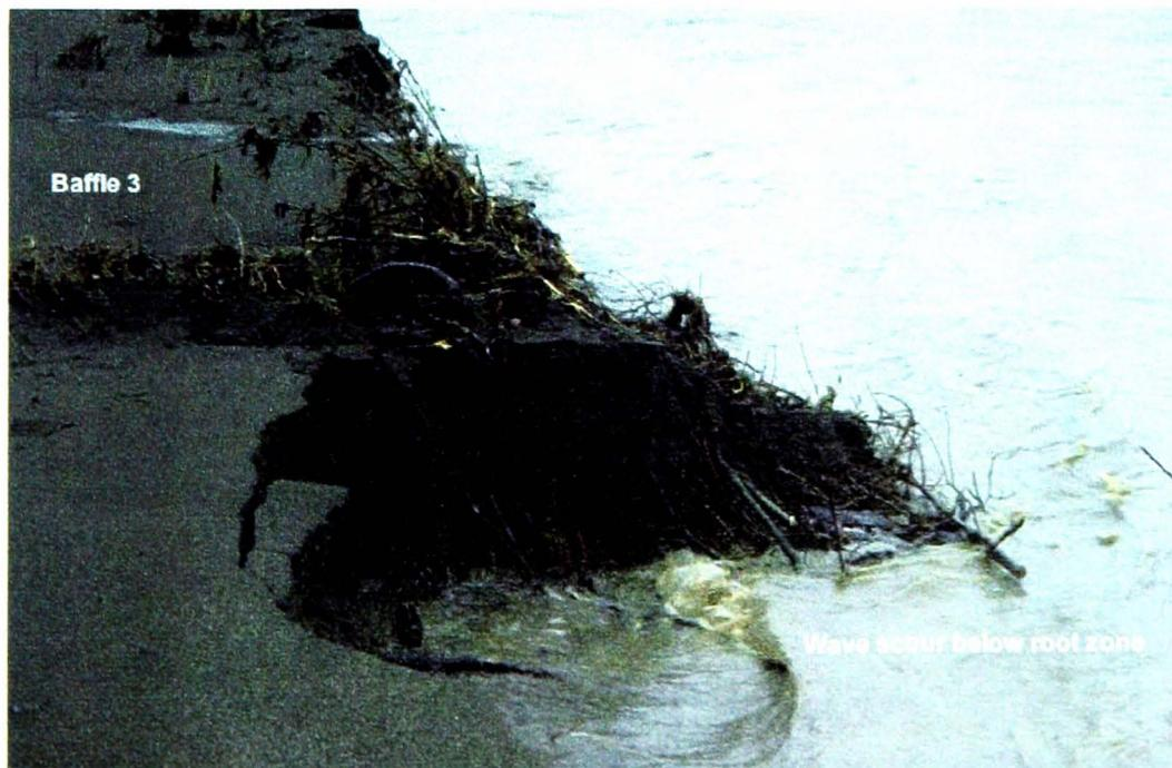
Photo 6.11. Calving bank and baffle eroding. Note wave scour below root zone occurring during flood recession 14 Jan 1995.
