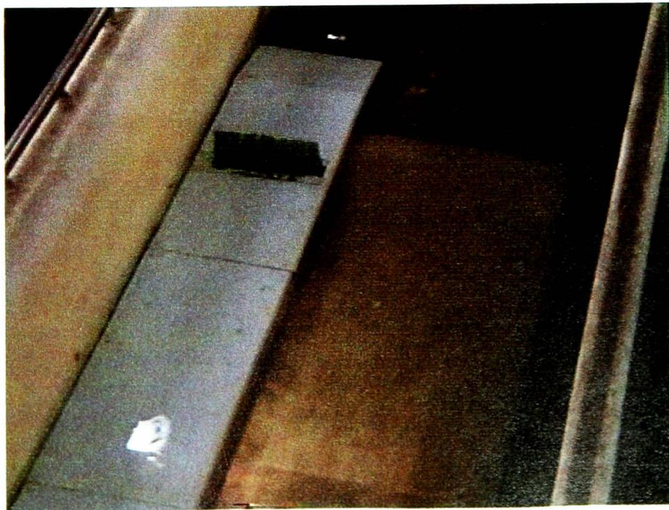
Photo 6.14. View of the final baffle design and simulated terrace in the flume.
