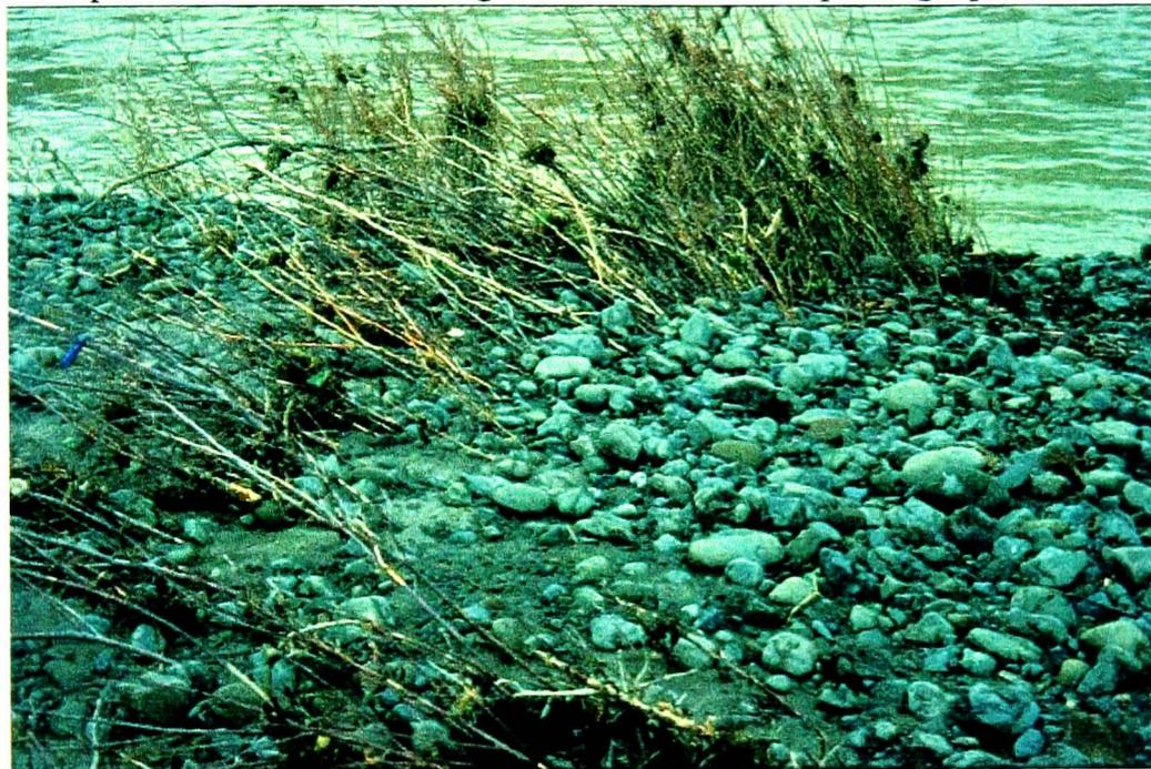
Photo 5.12. Sediment particles captured by baffles during 15 year flood, peak flow depth ~ 1m, photo taken 10 Jan 1995.
