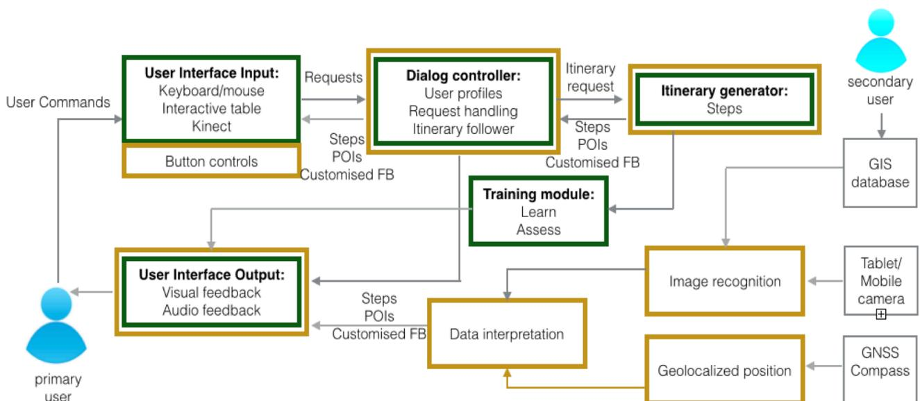
Figure 3. Main system modules
