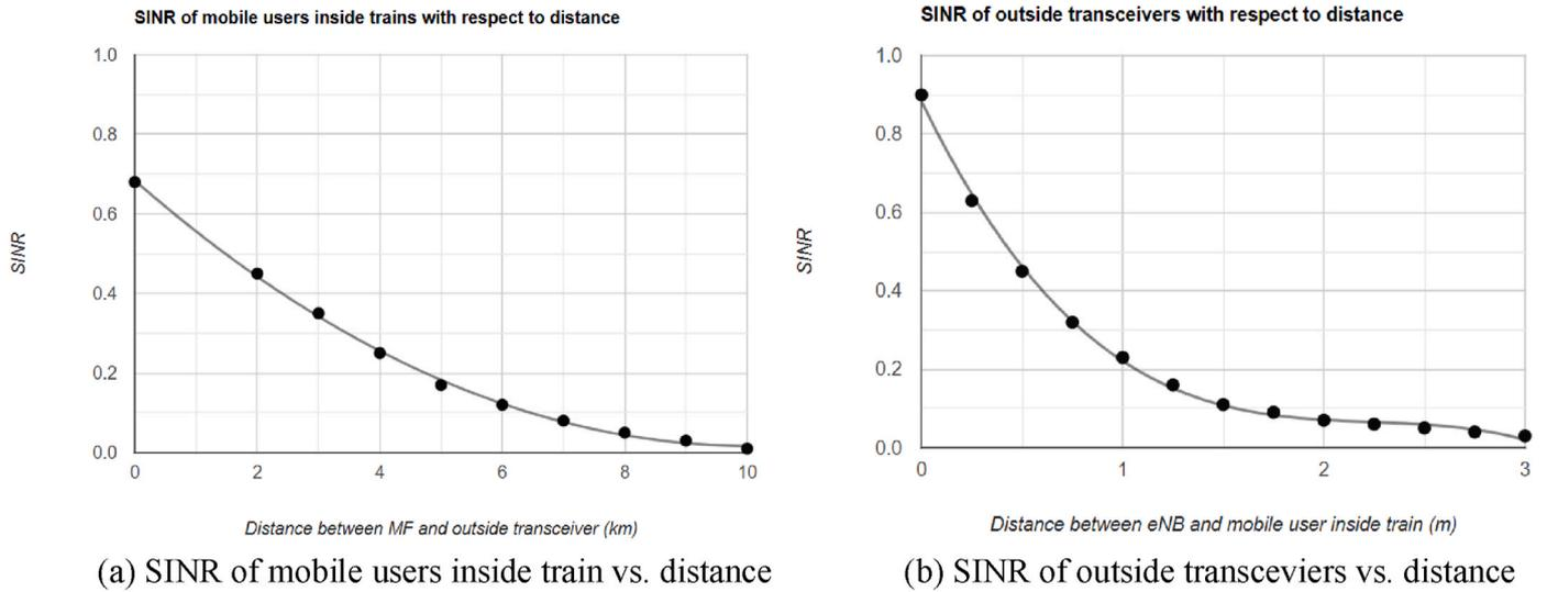
Fig. 7. (a) SINR of mobile users inside train vs. distance (b) SINR of outside transceivers vs. distance.
