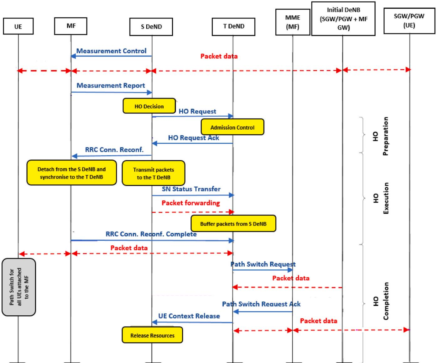
Fig. 5. Proposed HO mechanism for MF with its attached UEs.
