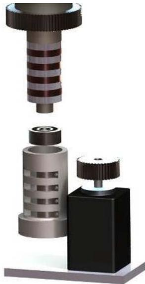
**Figure 7. Rotating connector mechanism**
