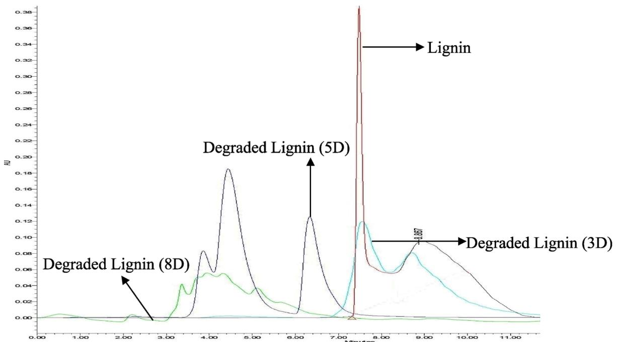
Fig. 7. Comparative HPLC chromatograph of control (lignin, 900 ppm) and lignin degraded by biofilm-forming potential bacterial strains.
