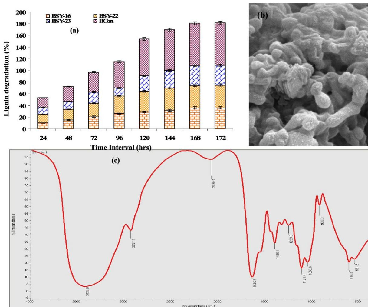
**Fig. 4. (a–c).** Showing lignin degradation by biofilm-forming potential bacterial strains (a), SEM view of consortium (b) and FTIR spectra of EPS extract (c) during lignin degradation.
