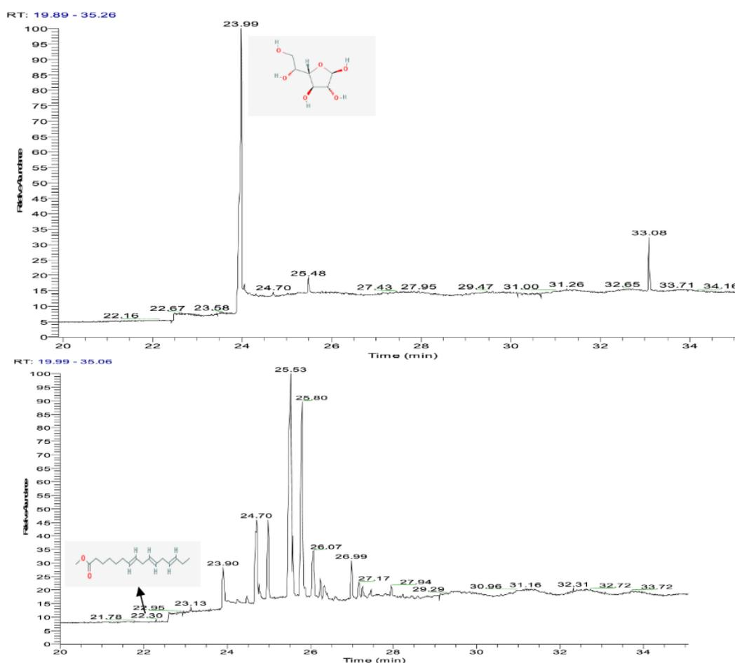
**Fig. 8.** Total ion chromatogram (TIC) of lignin as (top) control and (bottom) degraded lignin by biofilm-forming bacterial consortium.
