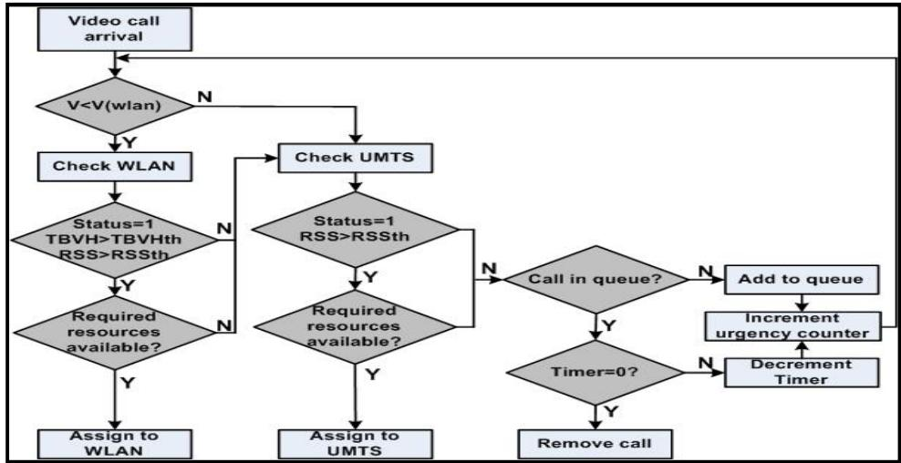
Figure 9. Application of TBVH in choice of networks
