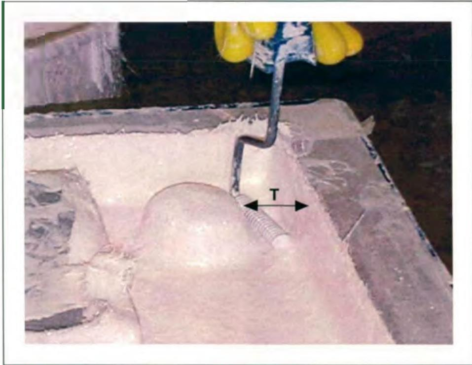
**Figure 32. Rolling task on a Pocket feature. Minimum tool-gap (T).**
