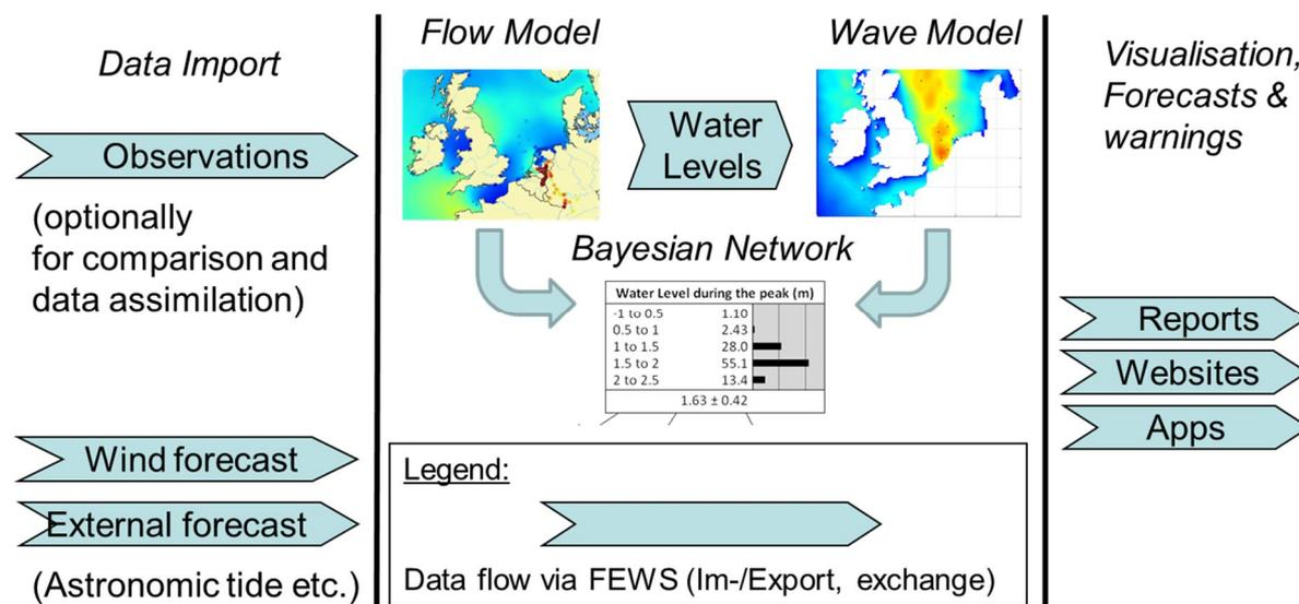
Figure 3. Schematic of Coastal Flood Early Warning System (EWS). Data imports are shown on the left. The physics-based and Bayesian Network models are shown in the middle panel and the visualisation and reporting output is shown on the right.
