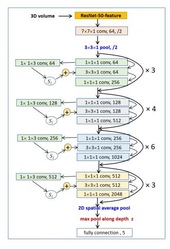
Figure 3. The depth-ResNet architecture applied in this paper, where ×N at each conv level refers to the block (e.g. conv5\_x) repeats N (e.g. 3) times consecutively.
