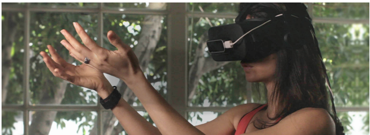
Figure 9: Leap Motion controller mounted to an HMD tracking hands and fingers (Leap Motion 2016a)
