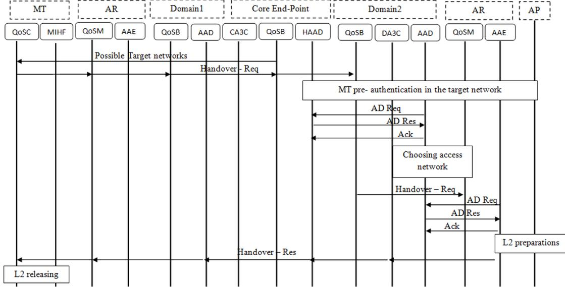
Figure 4.6: The Intra-Core End Point Handover Model
