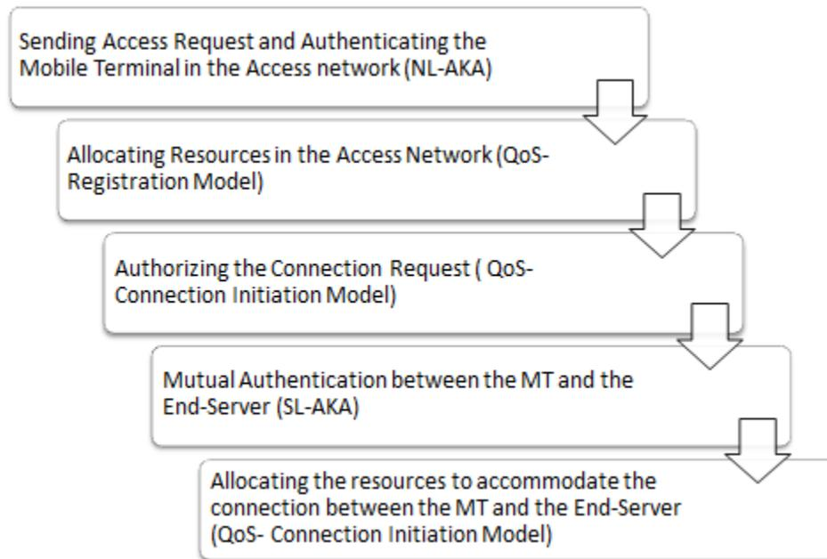
Figure 8.3: The Steps of Connection Security Model
