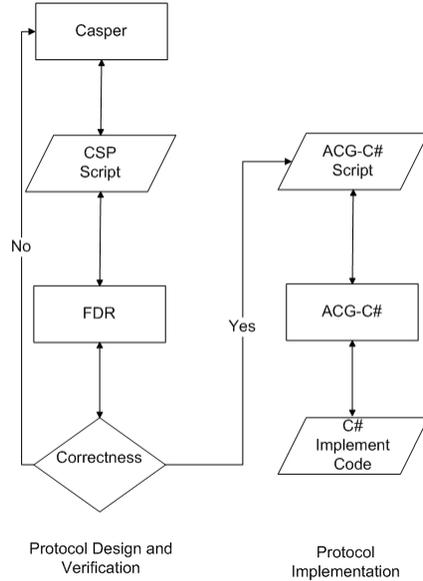
Figure 9.6: Security Protocol Design and Implementation (CJ05)
