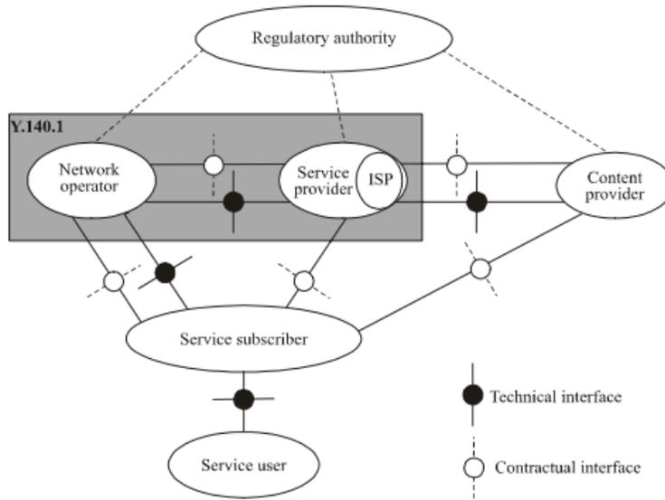
Figure 4.1: The ITU Recommended Network Parties
