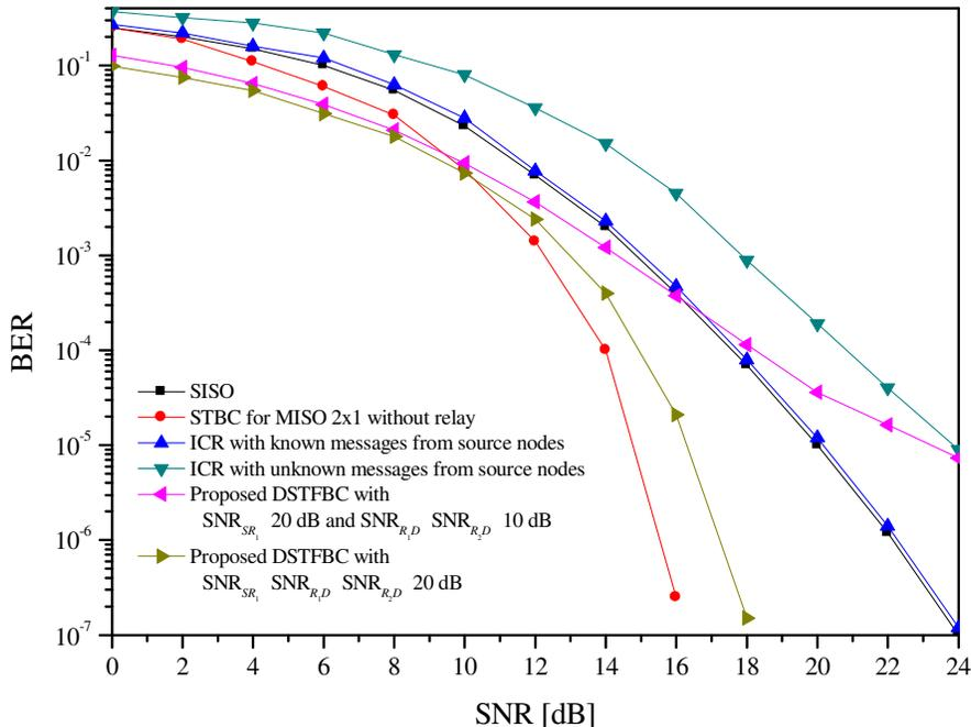
Fig. 3. Performance comparison of various transmission schemes in an CWBRN over Rayleigh frequency selective fading channels with  $L_{S_0\mathcal{R}_1} = 5$ ,  $L_{S_0\mathcal{R}_2} = 7$ ,  $L_{\mathcal{R}_1\mathcal{D}_0} = 5$ ,  $L_{\mathcal{R}_2\mathcal{D}_0} = 7$ .
