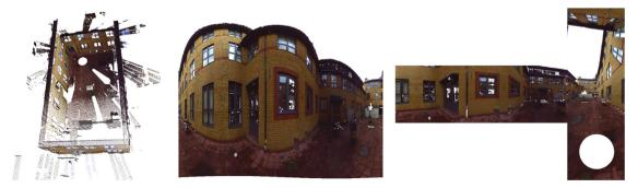
Fig. 5. Different representations of LiDAR data. Left: The 3D point cloud acquired from the LiDAR scan; Middle: A rendered spherical image taken from the location of the LiDAR scanner; Right: A rendered cubic image taken from the location of the LiDAR scanner.
