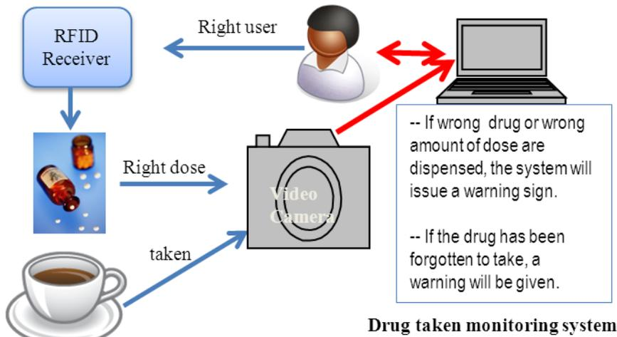
Fig. 2 Proposed system for monitoring medicine taking.
