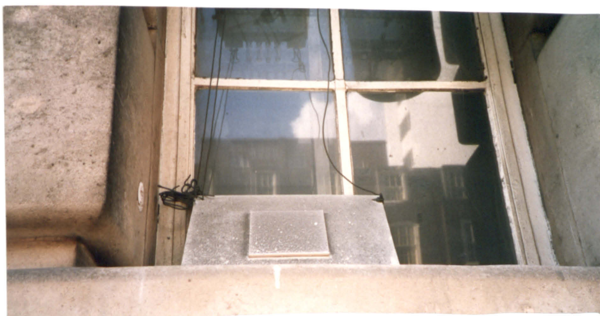
Figure 6.21 The experimental scheme used to display materials of tile and wood at a site on York Road, Waterloo, London. This photograph was taken after two months of exposure.
